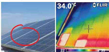
Defects in photovoltaic cells are clearly visible on a thermal image.
