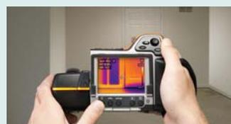
Infrared cameras quickly locate moisture related problems
